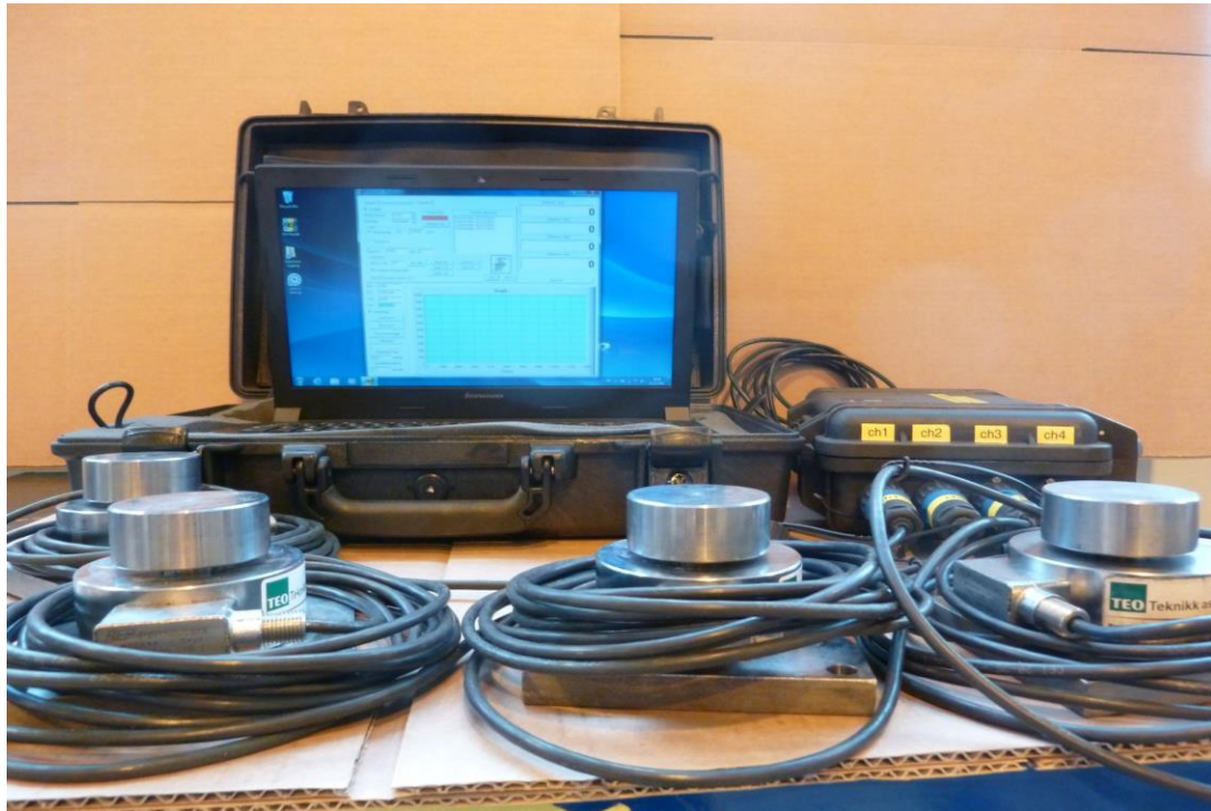
4 veieceller tilkoblet PC-logger/ 4 load cells connected to PC-logger.
